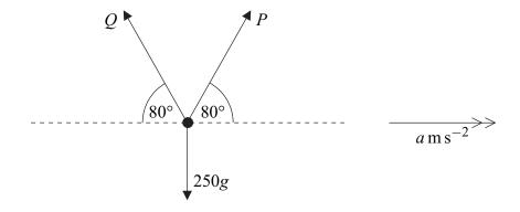
The two forces P newtons and Q newtons each act at  $80^{\circ}$  to the horizontal. The object accelerates horizontally at  $a \, \mathrm{m \, s^{-2}}$  under the action of these forces.
